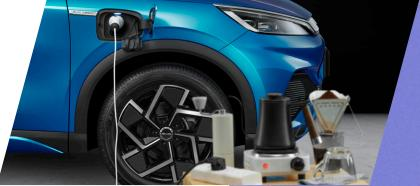
V2L (Vehicle to Load) function can connect 220V power from the car to supply other electrical devices.
